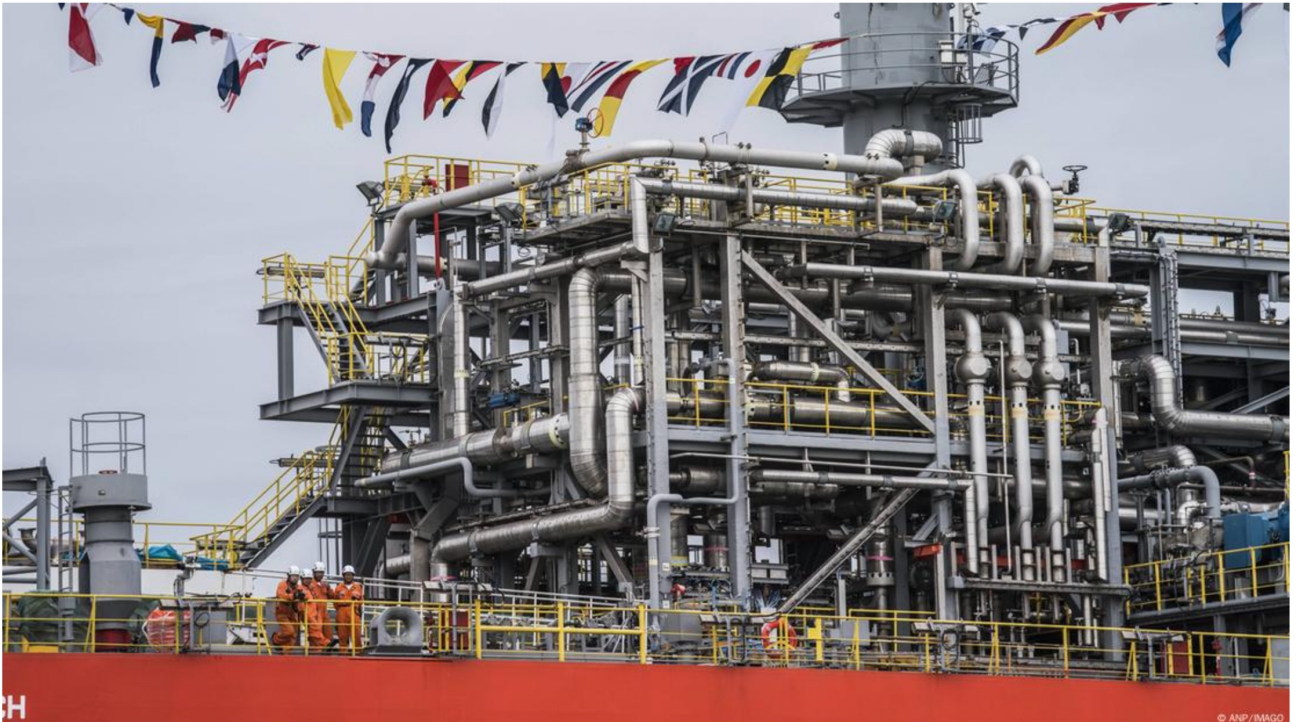
FSRUs (Floating Storage Regasification Units) are key infrastructures that facilitate the transportation of natural gas via sea
